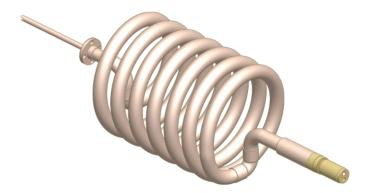
Drive thread is replaced, coil pitch is corrected, and all surfaces are reconditioned to ensure RF continuity.
